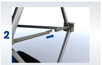
Lock all the lockers. Start at the outer edges and move towards the center.
