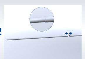
Assemble the two lower poles by inserting the upper pole into the plastic sleeve of
